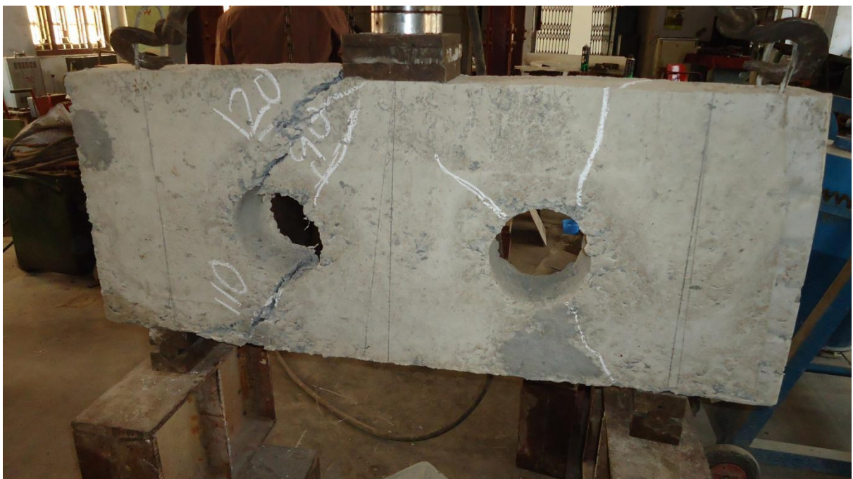
Fig. 4.7 Deep Beam specimen for testing
