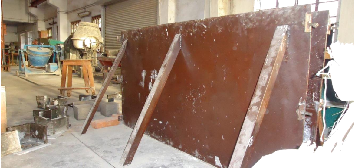
Fig.4.2 Deep beam frame
