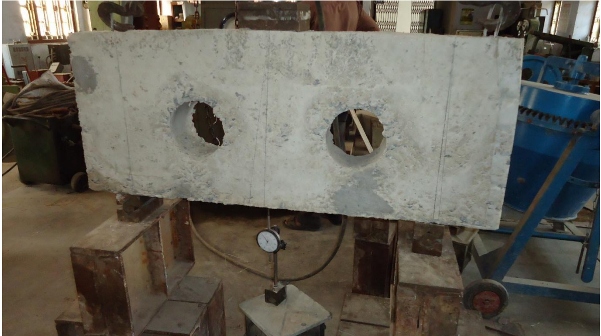
Fig. 4.7 Deep Beam specimen for testing
